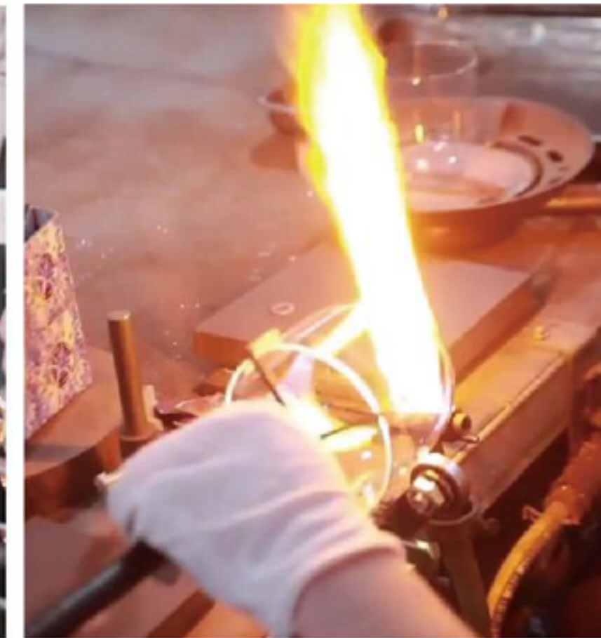
▲ 封底 Flatten bottom and prick hole
