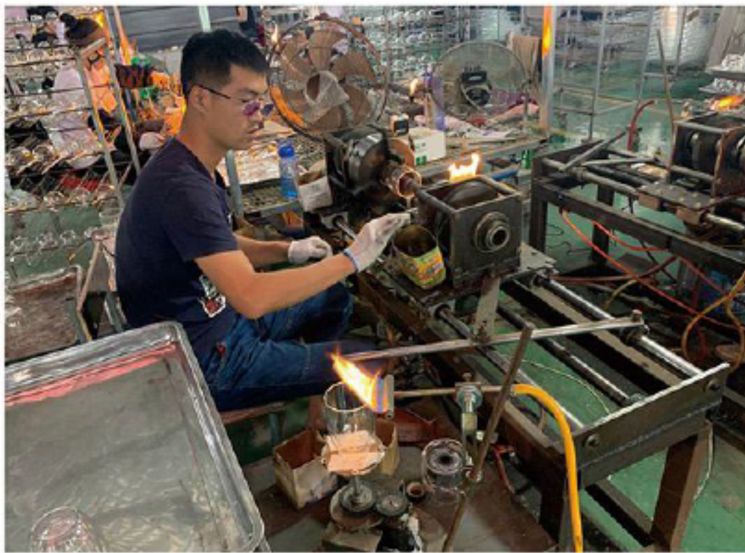
▲ 合口 Combining inner and outer body
