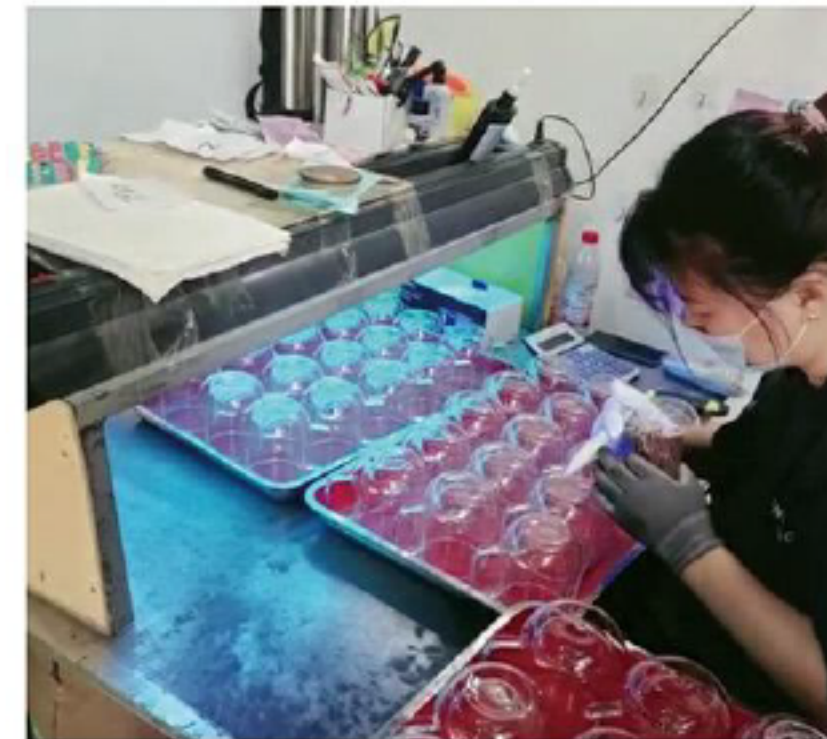
▲ 点胶 Bottom Hole Sealing (UV Lamp Box)
