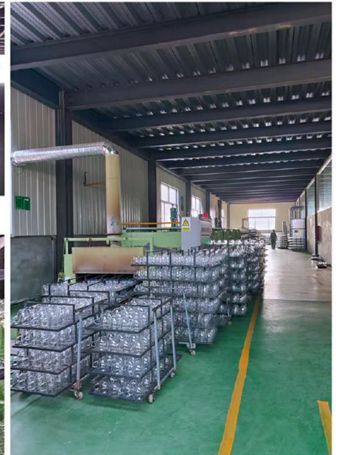
▲ 2号退火炉 No.2 Annealing Furnace
